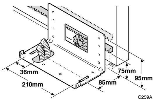
Install the rack at a height between 75 and 95 mm. 90 mm is recommended as the reference height.
